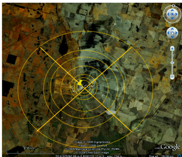
Figure 1. Soil sampling scheme for ecotoxicology study – 2009/2010. Sampling points are located where the concentric rings intersect the rays extending from the mining bund.
